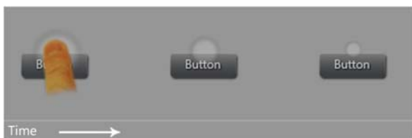
Fig. 11.14 Transition D (see Fig. 11.12): when contact is lifted, the visualization shrinks to the hit testing point. © 2009 ACM, Inc. Included here by permission
