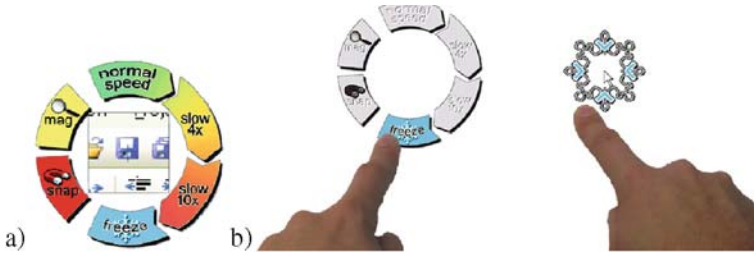
Fig. 11.9 Dual finger X-menu contains four selection areas for cursor speed control (normal, slow 4x, slow 10x and freeze), and two toggle areas (snap and magnify). Magnify mode presents an integrated magnification widget in the middle of the menu, while snap mode removes the current cursor offset. When freeze mode is selected, the cursor is completely immobile. © 2009 ACM, Inc. Included here by permission
